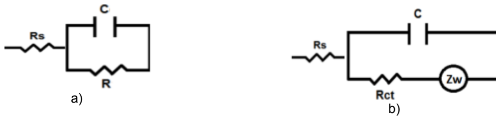
Figure 5 Common equivalent circuits used in impedance spectroscopy. a) Non-faradaic sensor b) Faradaic sensor. Adapted from [51].
